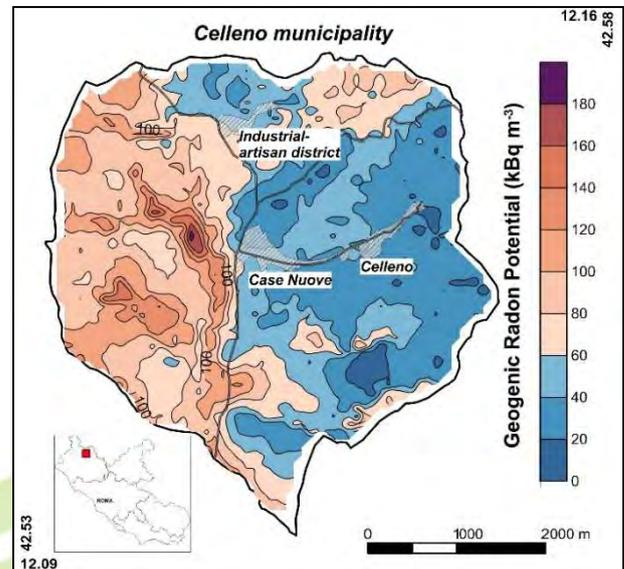
Figure 1. Geogenic radon potential map for the Celleno municipality (Giustini et al., 2019).
