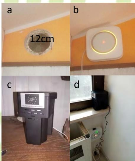
Figure 1. Respire Remediation System: a) SNAP must be installed on a wall in a 12 cm diameter hole that communicates directly with the outside; b) SNAP with working fan, the yellow light indicates that indoor radon concentration is below the reference level of 300 Bq/m<sup>3</sup>; c) RD2000M connected via Bluetooth with the SNAP; d) complete Respire Remediation System mounted in a school at Celleno municipality.
