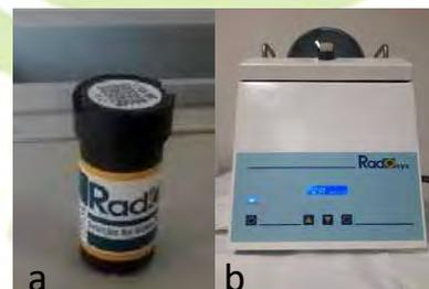
Figure 4. Radosys CR39 long-term indoor radon detector (a); automatic system for reading the alpha traces on the films of the exposed dosimeters (b).
