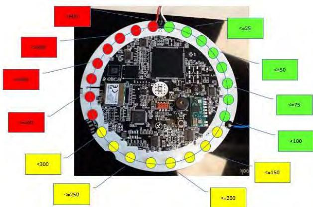
Figure 3. Photograph showing the series of LEDs that illuminate the outer ring, and the colors that change based on the measured Rn thresholds.
