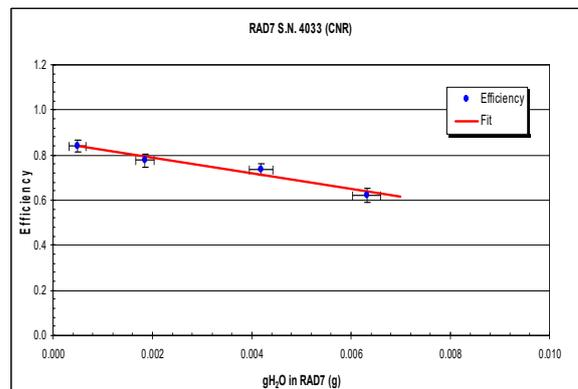
Figure 3. RAD7 S.N. 4033 (CNR) calibration. Efficiency trend as a function of  $\text{gH}_2\text{O}$  and linear data interpolation are shown.
